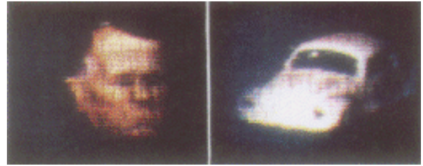
Figure 8: Two photographs of holographic images generated on our real-time holographic display. Left: polygonal model of head with texture-mapped face. Right: polygonal model of a car. View images for both objects were rendered in hardware at a resolution of 128×64.
